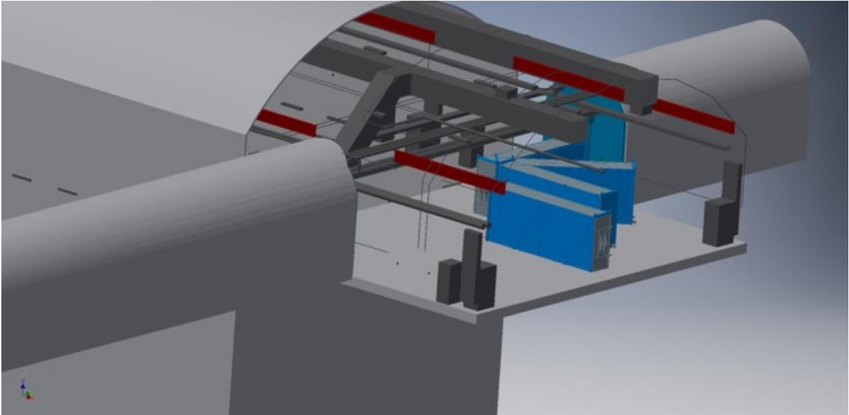
*Figure 3: Extraction of the current cavern model (exported from NX) containing ducting, piping and rails, which is then imported into AutoCAD Inventor. The APA transport boxes are added from the Far Detector models and work on understanding the installation motions has started*
