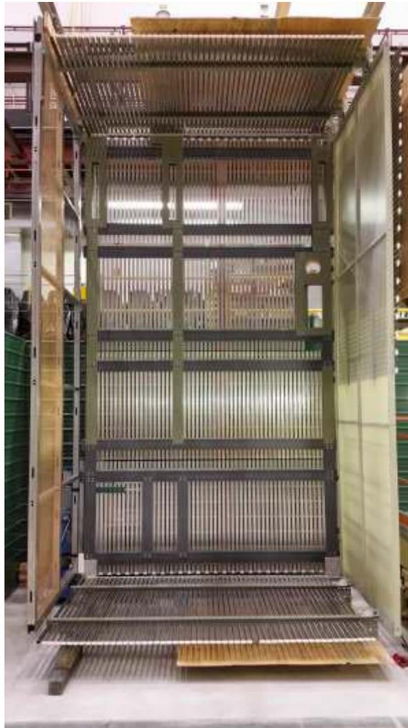
**Assembled ProtoDUNE-SP Field Cage, CPA and APA for Ash River Workshop**
