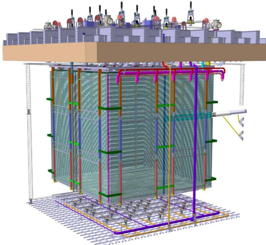
*Figure 1: Picture from the ProtoDUNE-DP design review. 3D view of the ProtoDUNE dual-phase detector integrated in the cryostat, including the penetrations in the cryostat roof, the cryogenic piping the cable trays in the cryostat corners and the corrugated membrane on the floor*
