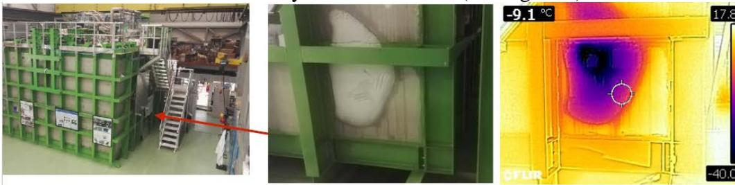
*Figure 1: Appearance of a cold spot with ice formation on the 3x1x1 cryostat exoskeleton during the cool-down procedure: details with visible light and infrared pictures*
