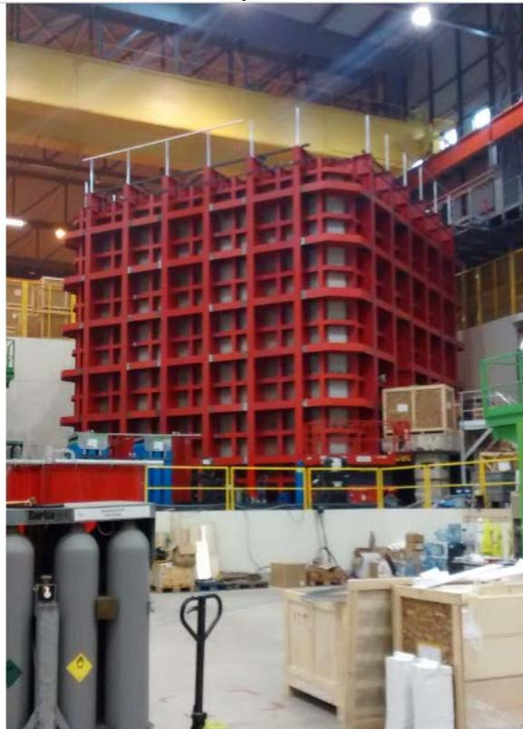
*Fig.5: Completion of ProtoDUNE-DP cryostat exoskeleton assembly.*
