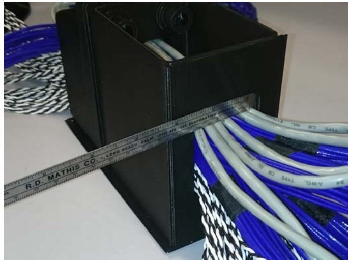
Figure 7: Photograph shows the cable bundle needed for the lower APA running through the corner of the APA side tube. It was not possible to fit all the photon detector cables through the opening and still have space for the link connecting lower and upper APA.
